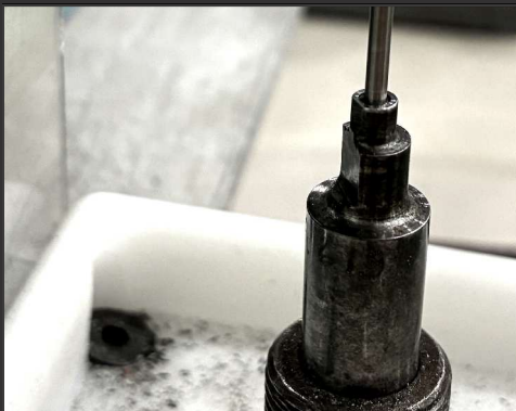
INHERITED CUSTOM ANVIL FAILED ON FIRST PRODUCTION ORDER
